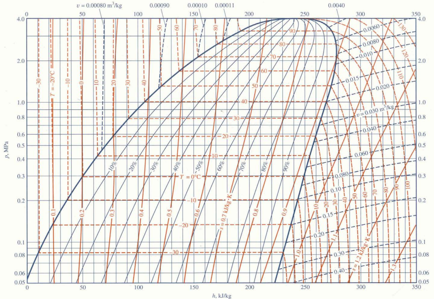
Chart A-11 R134a ph diagram. (Source: Based on Thermodynamic Properties of HFC-134a (1,1,1, 2-tetrafluoroethane) , DuPont Company, Wilmington, Delaware, 1993, with permission.)
